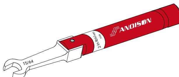
1. TORQUE VALUE:  $0.45 \pm 0.02 \text{ NM}$  [ $4 \pm 0.16 \text{ IN.LBS}$ ]
